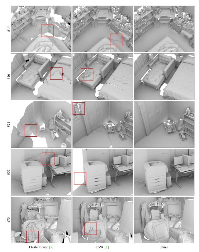
Figure 5. Reconstructions of five more scenes from the SceneNN dataset [2]. This extends Figure 3 in the paper. Prior systems suffer from inaccurate surface alignment and produce broken geometry. Our system produces much cleaner results.
