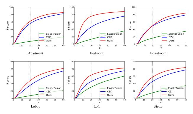
Figure 3. Accuracy of different reconstruction systems on the five scenes in the presented dataset, measured by F-score with varying distance thresholds  $\tau$  (in millimeters). The last plot shows the mean F-score for each threshold over all five scenes in the dataset.
